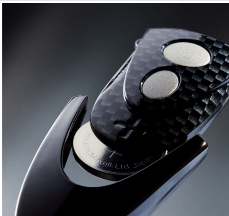
Handsender Micro-Novotron 512 Design 2-Kanal, 433 MHz, KeeLoq-Wechselcode
